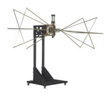
ETS-Lindgren's Model 3159C Biconical Antenna is a broadband, linearly-polarized biconical antenna. The 3159 Biconical Antenna exhibits a wide beamwidth and is specially designed to handle up to 10 kW input power for generating high electric field strength over a large uniform area.
