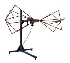
ETS-Lindgren's Model 3158 Biconical Antenna is a high power biconical designed for high level immunity. The Antenna can generate 100V/m over a ferrite covered ground at 2m distance per the ISO 11451-2 standard. The 3158 is a rugged version of the successful 3109 design. The 3158 has larger elements which reduce the VSWR at low frequencies. The rugged construction increases the power handling to 5 kW. It is a great antenna for generating higher fields in the 20 MHz to 120 MHz frequency band.
