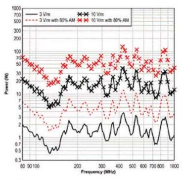
3143B BiConiLog Antenna Typical Average Power Required in Vertical Polarization at 3 m
