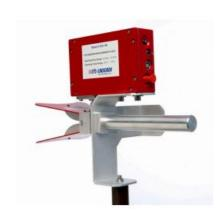
ETS-Lindgren's Model 3116C-PA is a special version of our popular Model 3116C Double-Ridged Waveguide Horn Antenna, fitted with a pre-amplifier package and calibrated as a single unit. By doing this, any possible mismatches between antenna and pre-amplifier are taken into account in the antenna factor (AF), which is provided with this unit.
