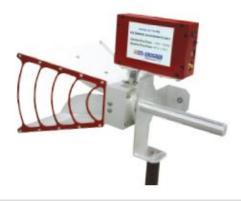
ETS-Lindgren's Model 3115-PB is our popular Model 3115 Double-Ridged Waveguide Horn Antenna, fitted with an updated pre-amplifier package and calibrated as a single unit. In this configuration, any possible mismatches between antenna and preamplifier are taken into account in the antenna factor (AF) which is provided with this unit. Please note, the 3115-PB is not intended for RSE testing of intentional radiators.
